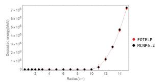
Figure 3. Comparison of deposited energy in concentric spheres for 10 MeV using FOTELP and MCNP codes
