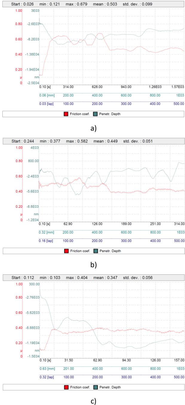
Figure 2. Coefficient of friction and Penetration depth plots for 240p grit size Aluminium sample under three sliding speeds: a) 1mm/s, b) 5mm/s and c) 10mm/s.
