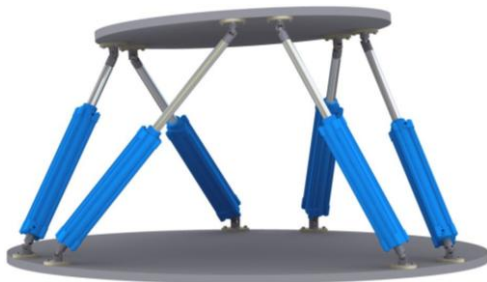
Fig.1. A 3D model of a 6-DOF parallel robot platform
