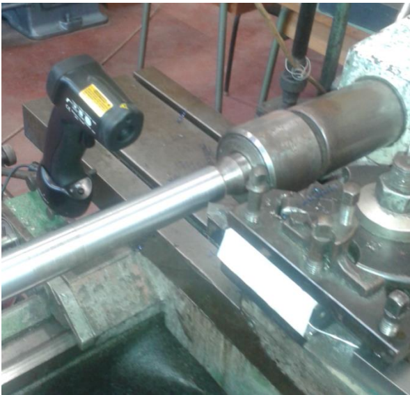
Figure 7. Position of the turning knife and IR thermometer during longitudinal turning
