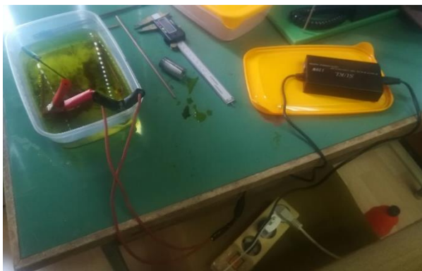
Fig. 1. ESM of a circular cross-section specimen with non-standard dimensions
