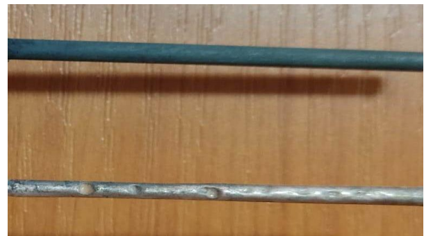
Fig. 3. Dimensional errors and surface defects of specimen made by ECM using 48V voltage
