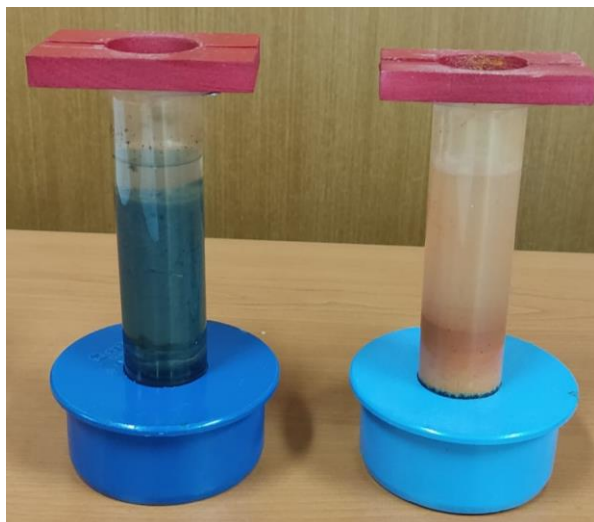
a) b) Fig. 5. The appearance of the electrolyte after processing depends on the type of processed material a) steel; b) brass
