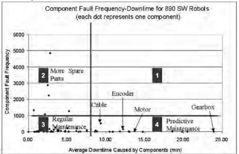
Figure 2 - Four qvadrant chart for identifying critical components
