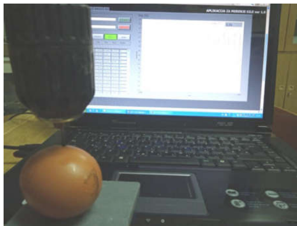
Slika 1. Uređaj za merenje sile probijanja ljuske jaja Figure 1. Device for measuring puncture force of egg shell
