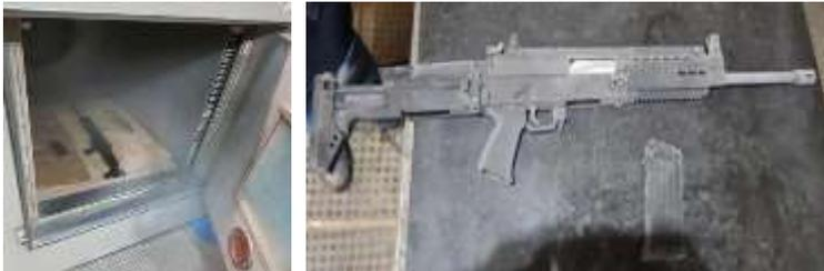
**Fig.4.** Inserted ammunition frame and the rifle into the chamber – left, frame ammunition and rifle after reaching the temperature of -30 °C
