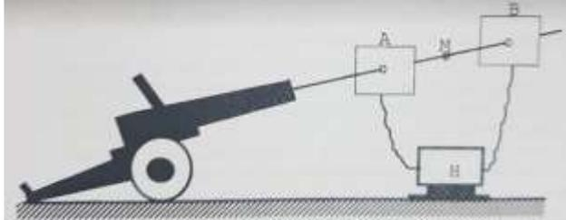
**Fig. 2.** Method for measuring the projectile's initial velocity [7]
