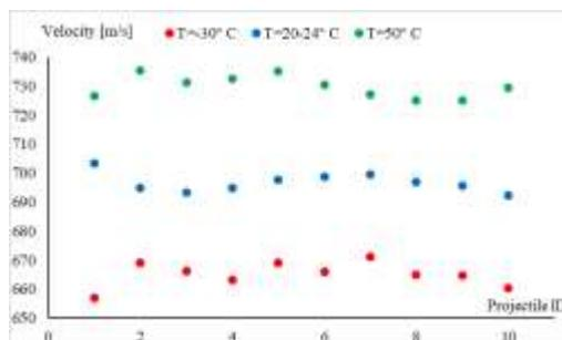
**Fig. 7.** Projectile velocity
