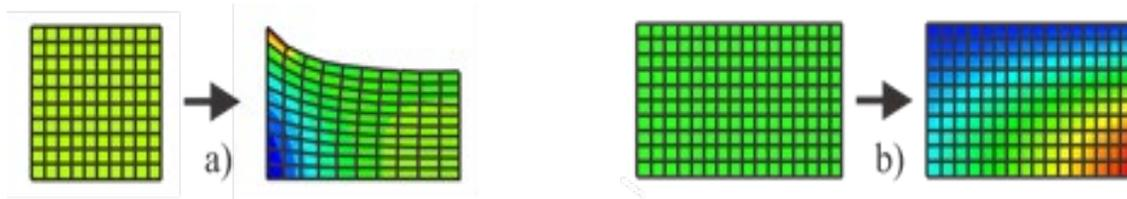
**Fig. 1.** Numerical formulations: a) Lagrangian b) Eulerian
