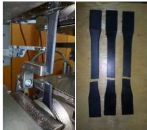
Fig. 5. Broken specimen in the machine grips (left) and three specimens after tensile test (right)
