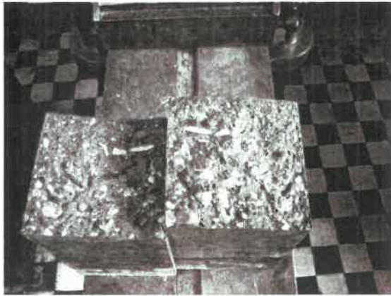
Slika 15. Lom po cementnoj pasti Figure 15. Fracture at cement paste
