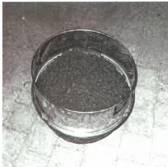
Slika 13. Test na situ Figure 13. Sieve segregation test
