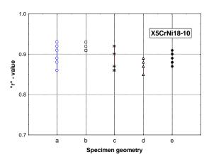
Fig. 14. "r"-value dependence on specimen geometry (X5CrNi18-10)
