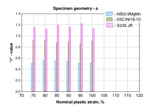
Fig. 19. "r"-value dependence on nominal plastic strain
