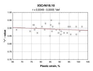
Fig. 11. "r"-value dependence on plastic strain (X5CrNi18-10)
