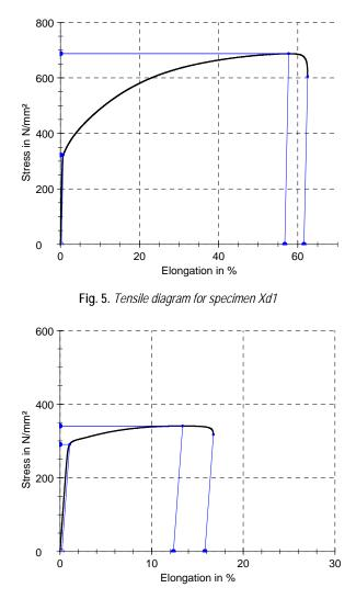
Fig. 6. Tensile diagram for specimen Ad1
