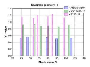
Fig. 18. "r"-value dependence on real plastic strain
