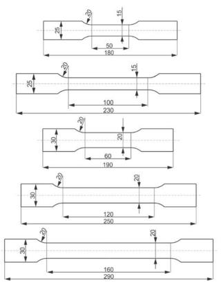
Fig. 2. Geometry of test specimens
