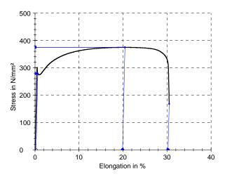
Fig. 4. Tensile diagram for specimen Sd1
