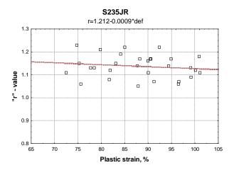
Fig. 10. "r"-value dependence on plastic strain (S2235JR)
