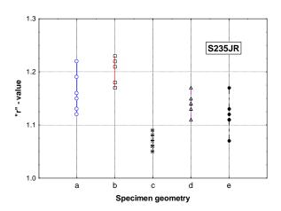
Fig. 13. "r"-value dependence on specimen geometry (S235JR)
