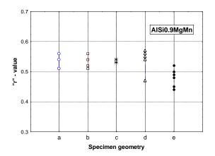
Fig. 15. "r"-value dependence on specimen geometry (AlSo0.9MgMn)
