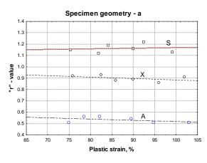
Fig. 16. "r"-value dependence on plastic strain
