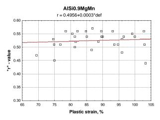
Fig. 12. "r"-value dependence on plastic strain (AlSi0.9MgMn)
