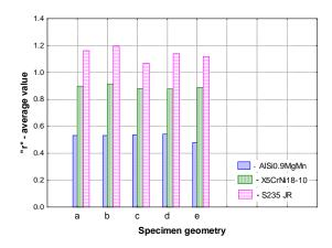
Fig. 17. "r"-average value dependence on specimen geometry
