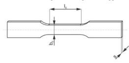
Fig. 1. Uniaxial tension test specimen
