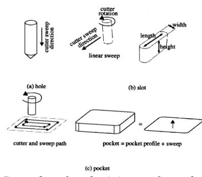
Figure 5: Procedure for obtaining surfaces during processing
