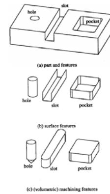
Figure 4: Basic shapes of surfaces on the workpiece
