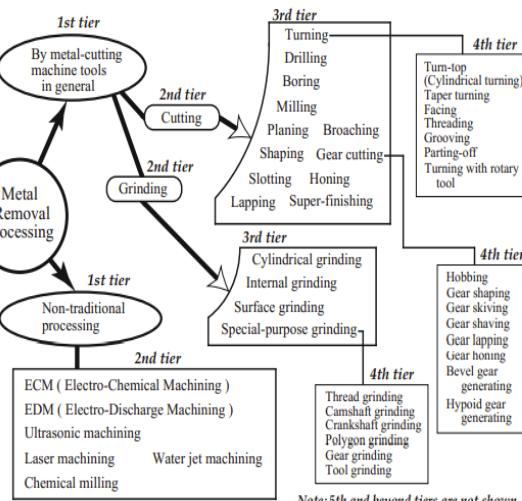
Figure 1: classification of different types of metal processing
