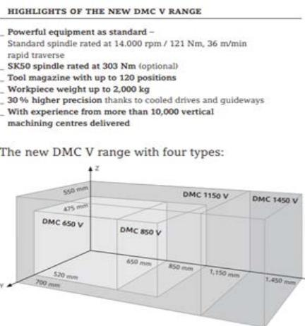
Figure 3: Dimensions of the workspace different types of machining centers from Deckel Maho DMC
