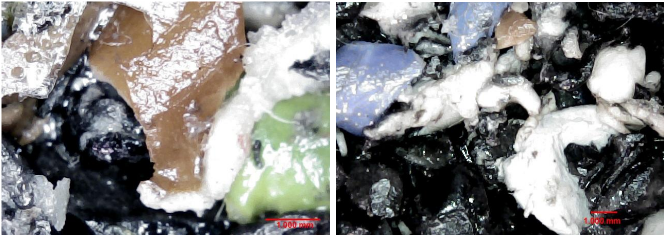
Fig. 2 Enlarged view of the structure of the granulate from recycled plastic
