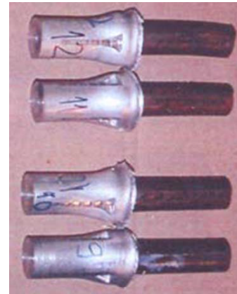
Figure 2. Technical drawing and physical appearance of samples (a) and welded Al-Cu samples (b)
