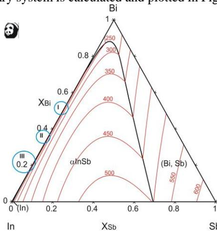
Fig. 1. Calculated liquidus surface of the ternary Bi-In-Sb system
