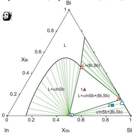
Fig. 5. Isothermal section of the ternary Bi-In-Sb system at 400°C and experimental values of the
