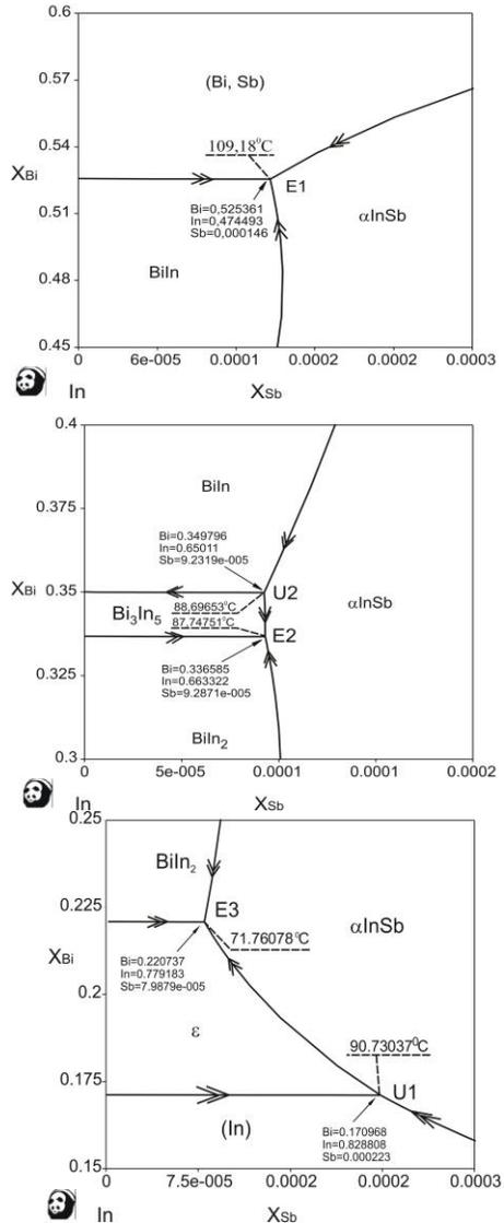
Fig. 2. Magnified views of the liquidus surface projection of Bi-In-Sb ternary system in a vicinity of : I ) E1 eutectic point; II ) E2 eutectic point; III ) E3 eutectic point
