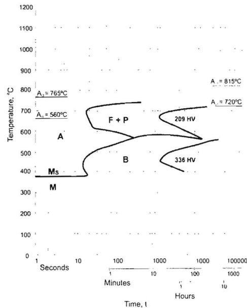
Fig. 3 CCT diagram for 25CrMo4 steel
