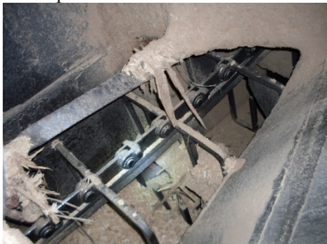
Sl. 4. Lančani transporter sirove strugotine
