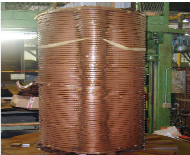
Fig. 13 Deformation of windings due to short circuit
