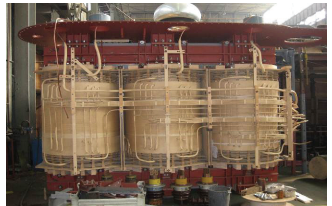
Fig. 11 The active part of power transformer
