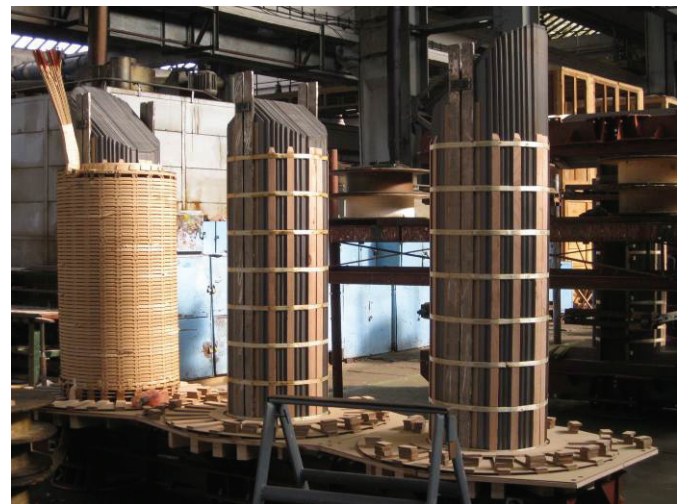
Fig. 7 Tighten pillars of magnetic core with yoke being taken off in the assembly process
