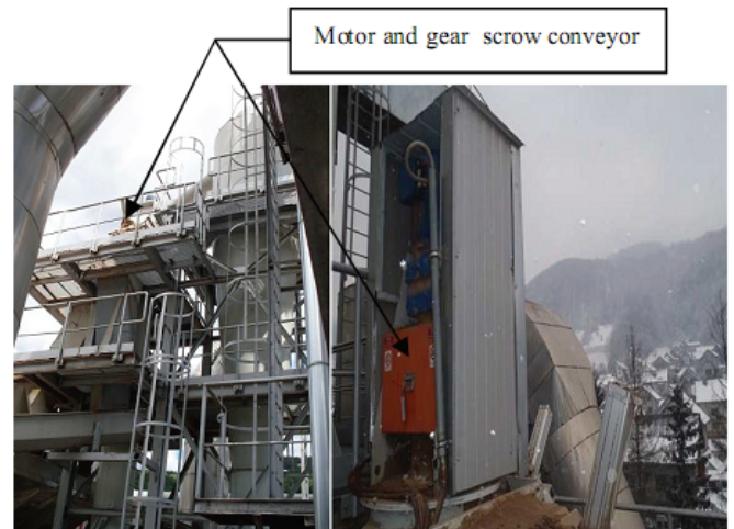
Fig. 9 Vertical worm transporter – before and after sound protection
