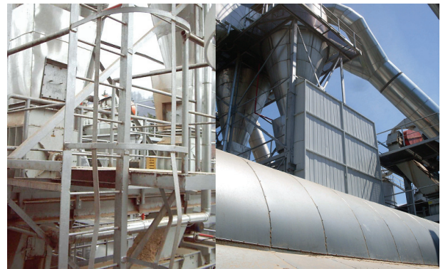
Fig. 10 Inter layer halts – before and after sound protection
