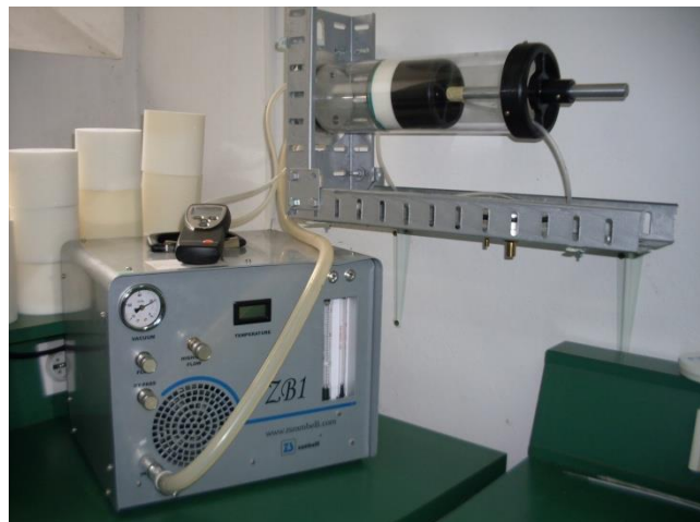
Fig. 6 Look of the realized measurement system for determination of airflow resistance
