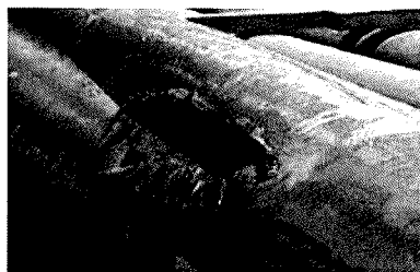
Fig. 1 General corrosion of well pipes and pipeline failure [1]
