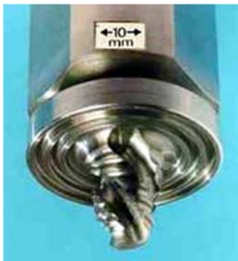
Fig.4 Tool for FSW process with three spiral flutes [6]
