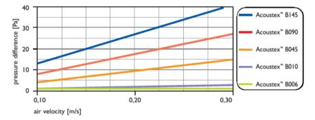
Fig. 8 Dependence of the pressure drop for different types of materials (www.satiamericas.com)
