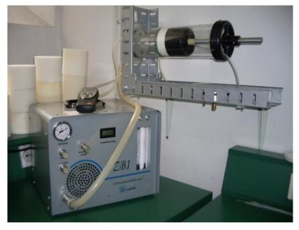
Fig. 6 A view on the realized measurement system for determination of airflow resistance
