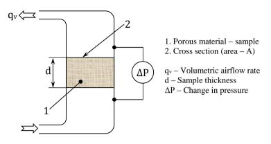
Fig. 3 Steady-state method (method – A) – Basic principle
