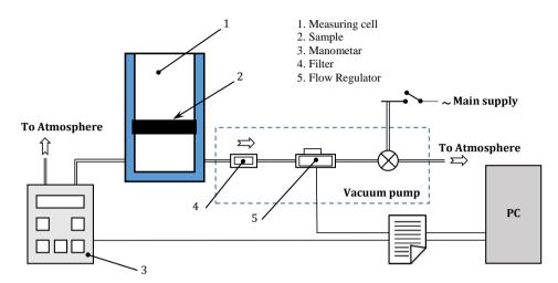
Fig. 5 Block diagram of the steady-state airflow system
