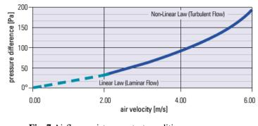
Fig. 7 Airflow resistance – test conditions: linear and non-linear (www.satiamericas.com)
