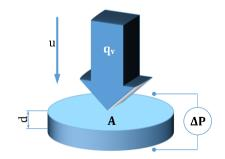
Fig. 2 Schematic presentation of measuring airflow resistance
