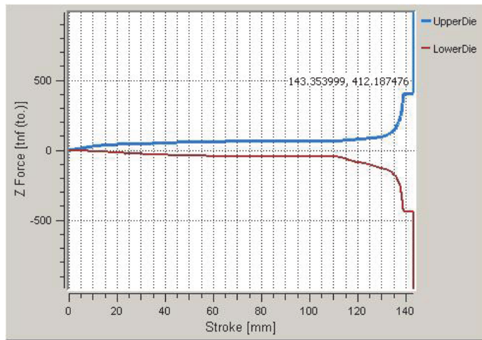
Fig. 9 Dependence of forging force on stroke
