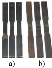
Figure 2 [1] Prepared samples for tensile test BM a) and welded joint b)
