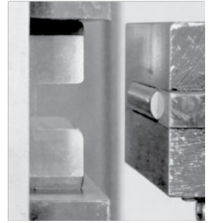
Fig. 6. Drawbead and die in contact
