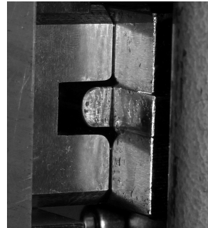
Figure 6: Drawbead and die in contact.
