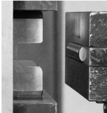
Figure 5: Drawbead and die before contact.
