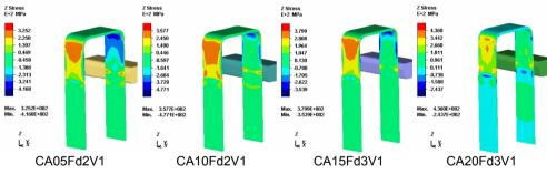
Figure 11: Axial stress distributions at ironed strip during ironing process
