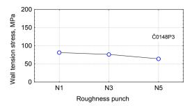
Figure 9: Average values of the wall tensile stress for various punch roughnesses.
