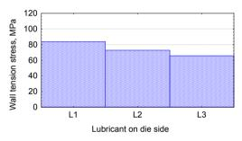
Figure 7: Average values of the wall tensile stress for various lubricants on the die.
