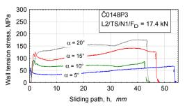
Figure 5: Variation of the wall tensile stress with the sliding path for various die slope angles.
