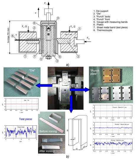
Figure 2: Scheme (a) and appearance of the model (b) used in this investigation.
