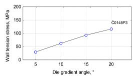
Figure 6: Variation of the wall tensile stress with the die slope angle.
