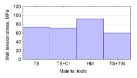
Figure 8: Average values of the wall tensile stress for various tool materials.
