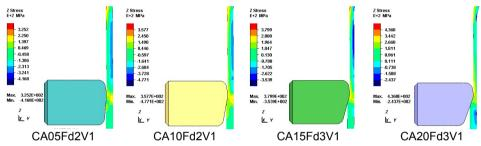
Figure 10: Wall stress distributions in numerical FE experiments of ironing.
