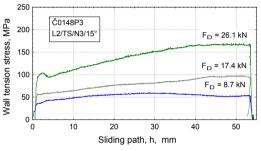
Figure 3: Variation of the wall tensile stress with the sliding path for various holding forces.
