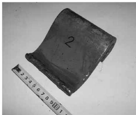
Fig. 12. Appearance of the hard faced knife
