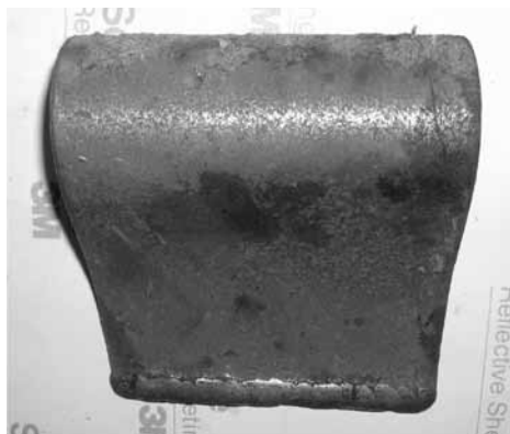
Fig. 13. Appearance of a knife hard faced by grinding
