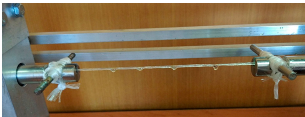
Figure 3. The twine sample prepared for testing (previously immersed in oil and prestressed by twisting).
