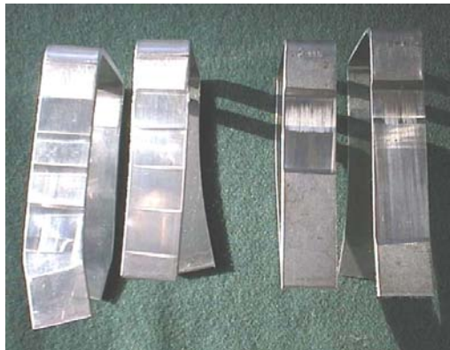
Figure 10: The appearance of test-pieces after multistage drawing
