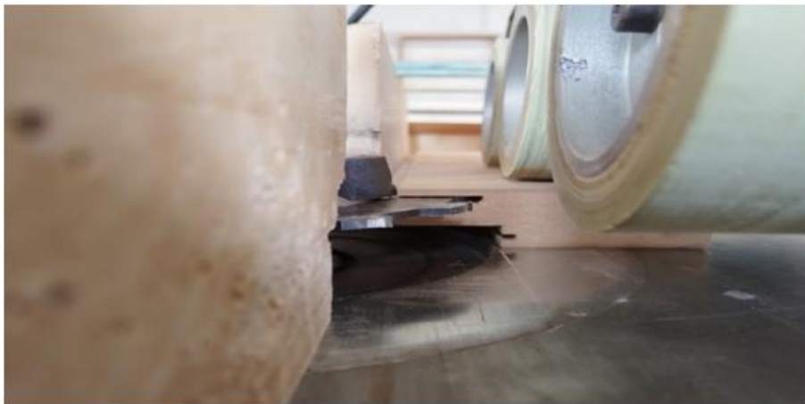
Fig. 10 Tool adjustment using a template
