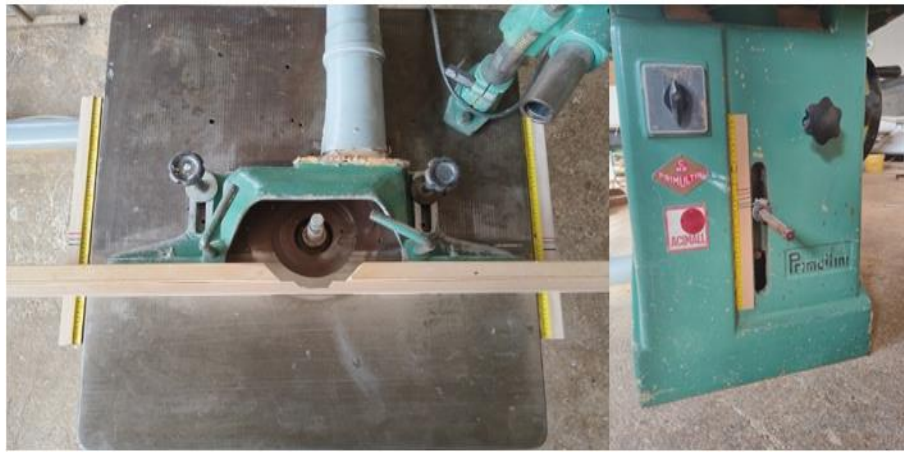
Fig. 11 Tool adjustment by width and height
