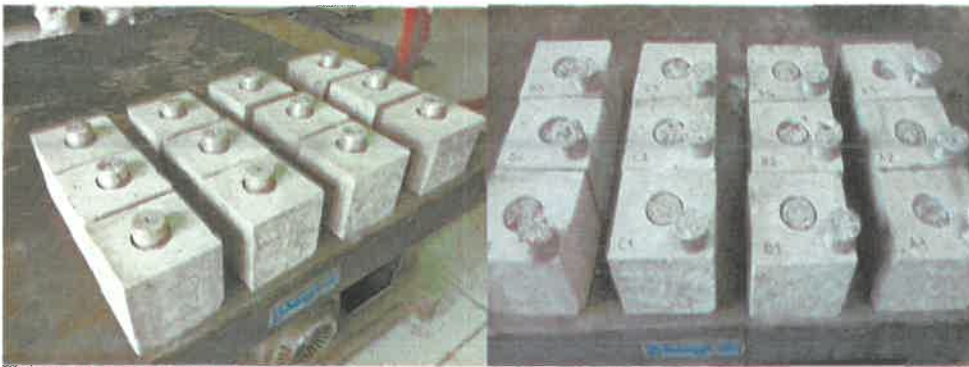
Figure 3. Specimens before and after the Pull-off test
