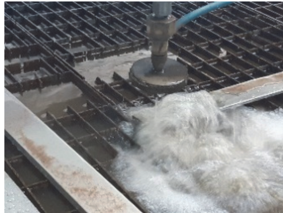
Figure 4: Cutting head of the PTV-3.8/60 machine during sample cutting
