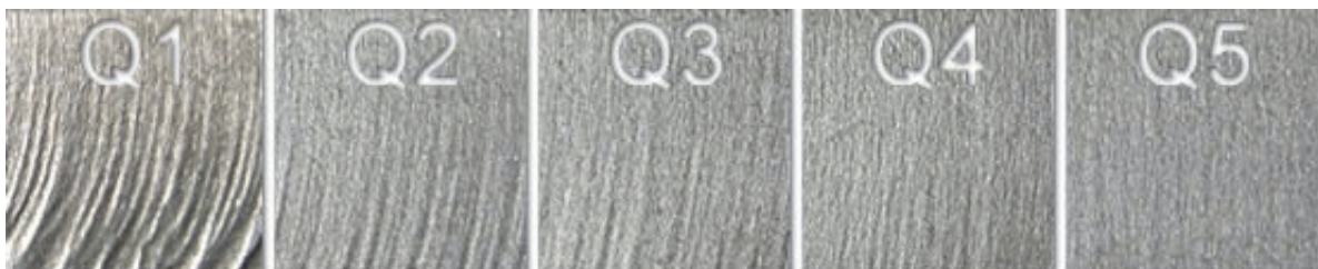
Figure 2: Five characteristic qualities of the machined surface [2]
