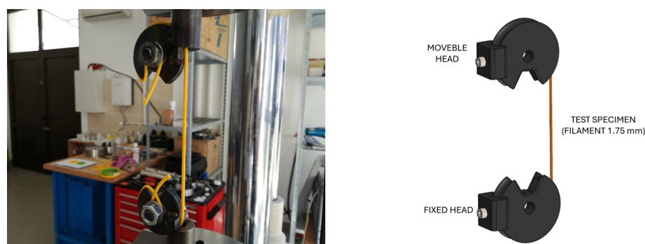
Figure 4. Uniaxial tensile testing of filament procedure: (left) equipment for uniaxial filament testing and (right) sketch of equipment.
