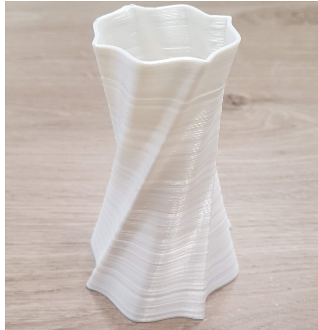
Fig.12. Test part printed during the testing phase of the 3D printer
