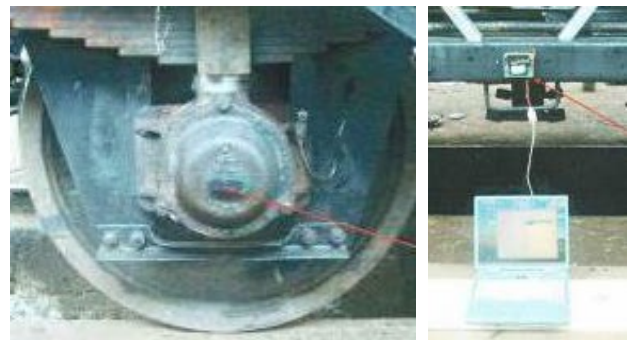
Fig.8. Preliminary tests of system for on-line monitoring of axle-boxes temperature
