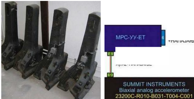
Fig.5. Instrumented autocouplers Fig.6. Block diagram of system for car body acceleration measurement
