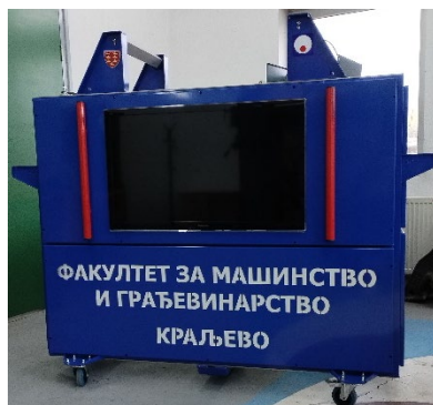
Fig. 12. Test stand for bridge models testing
