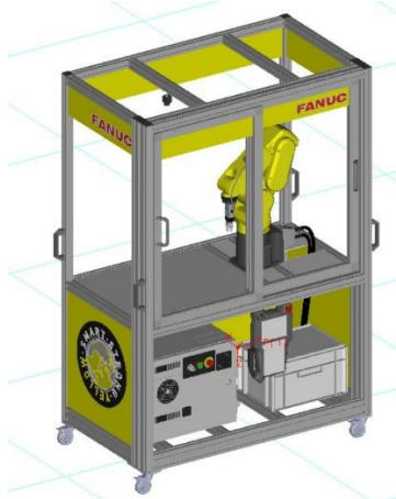
Figure 1. 3D model of FANUC educational cell
