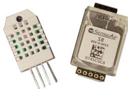
Figure 8. Used temperature/humidity sensor (left) and CO 2 sensor (right)
