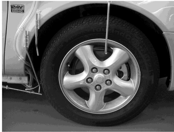
Figure 2 Image of test vehicle showing location of sampling tubes [2]
