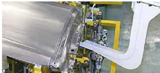
Figure 11 Application of FSW for rear doors on the Mazda RX-8 [11]
