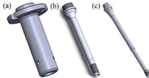
Figure 7 FSSW tool components: a) clamping ring, b) sleeve, c) pin [9]
