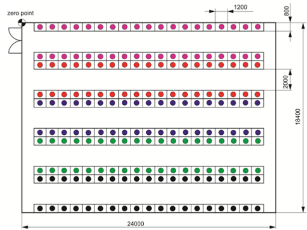
Fig. 2. Layout of a high-bay warehouse with associated dimensions and materials (• wood, • cardboard, • chipboard, • PVC, and • rubber)
