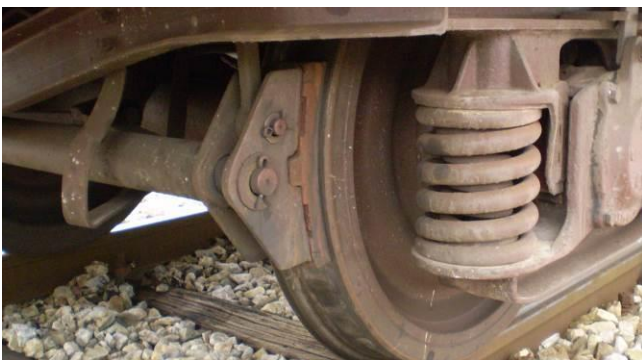
Fig.1. Braking elements of freight wagon
