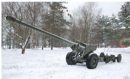
Figure 1. View of the 130 mm M46 gun [2]
