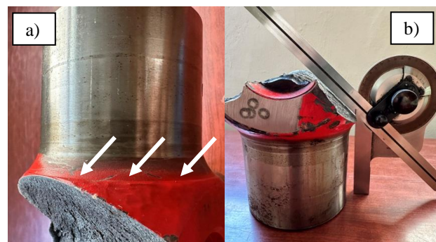
Figure 2.2. Fracture of the sleeve of the UCJ
