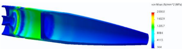
Figure 8. Stress condition for a model with 13 kg propellant charge
