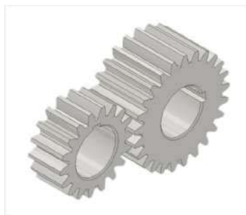
Fig. 5. Model of gears with 18 and 25 teehts
