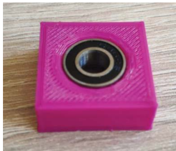
Figure 3 Appearance of the press-fitted bearing assembly within the 3D-printed housing
