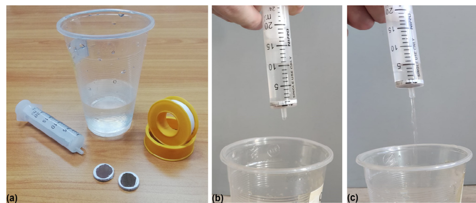
Figure 4. Custom setup for water flow tests: (a) water container, test samples, syringe, PTFE tape; (b) suspended water flow with the sample with a non-porous structure (Figure 3b); (c) water flow through a filter with a porous structure (Figure 3a).
